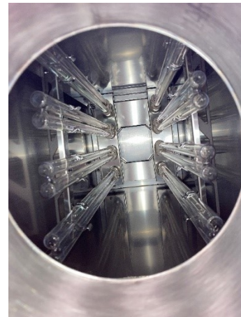
Picture 2: UV-C-lamps – reactor chamber
